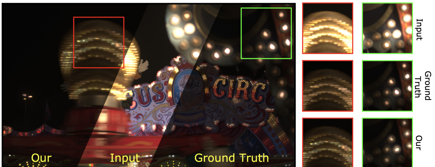
An example of our inverse tone mapping operator applied to an SDR version frame from the Carousel fireworks 02 sequence [13]. Our method can recover missing texture, colors, and dynamic range details in a convincing way.
